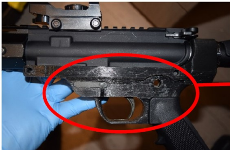
'Polymer 80' Glock frame with factory slide and prohibited 'auto-sear' (converts pistol to full automatic)
